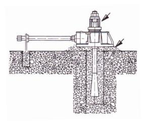
Remove the clamping sleeves when the grouting in the centre rows has set.
