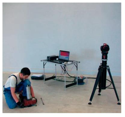
Each BW-Fixator® will be set individually into the reference coordinate system. Thus, there are no subsequent errors.
